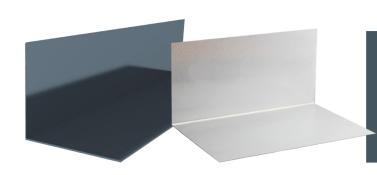
Aluminium soakers are for use when forming a pitched roof against an existing wall. Pre-fabricated to a 90 degree angle, soakers are inserted between successive courses to make a waterproof joint. A lightweight and durable alternative to lead.
