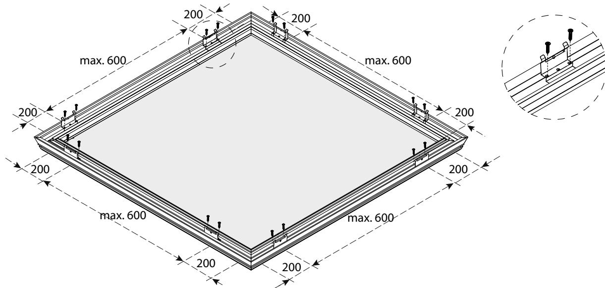
Turn around the complete system and put it above the curb! Make sure the clips, the complete system of window and glass, are not directly placed on the roof covering or underground (to avoid damage on the roof covering or clips). Present the frame on the curb and divide the play equally over the 4 sides of the curb. Simply push the frame over the curb to clip the frame on the curb.
