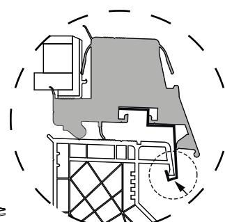
For extra reinforcement, screw the clips through the curb with delivered (one-way) screws.
