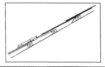
Roof void ventilation slate with free vent area of 10,000mm<sup>2</sup>.
