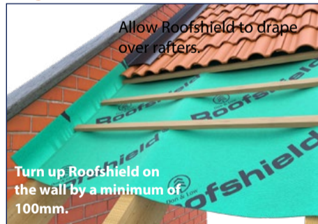
Verge Abutment Detail
